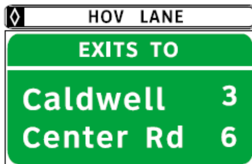
Figure 16. Distance / Destination Sign example from TxDOT Managed Lanes Guidelines. (Note: Example shows sign for a traditional HOV lane as indicated in the banner).
