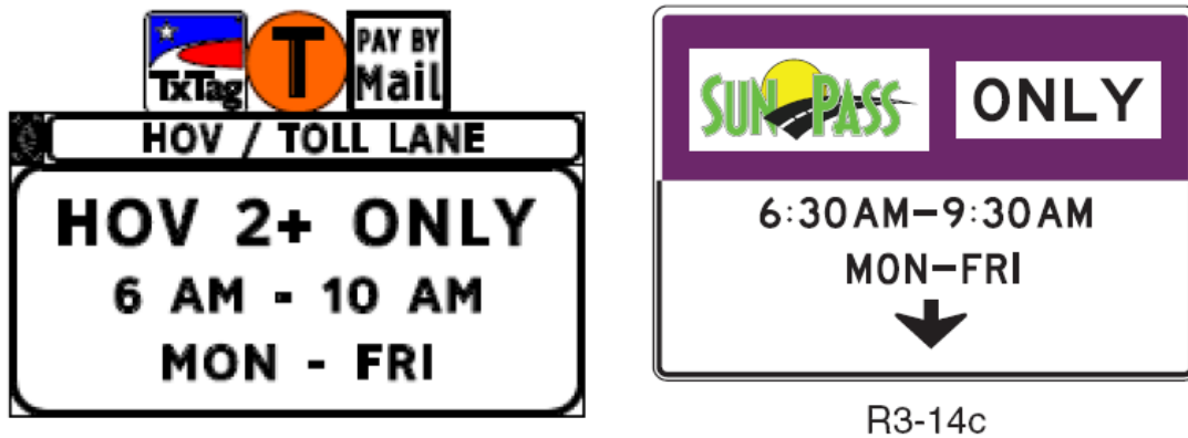
Figure 24. Example regulatory signs from the TxDOT Draft Guidelines (left) and the Federal NPA (right).
