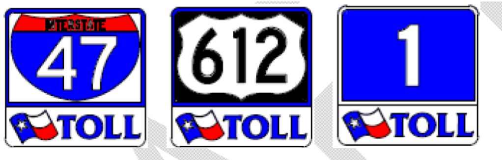
Figure 18. Toll route markers from the Texas MUTCD
