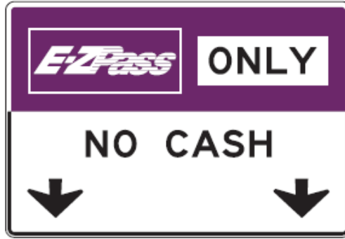
Figure 2. NPA Figure 2B.9, Example of R3-16 regulatory sign for ETC lanes at a conventional toll plaza, with adjacent cash lanes.
