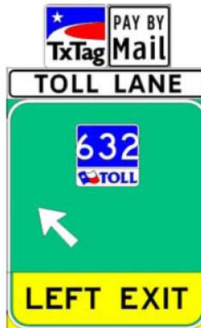
Figure 20. Example sign from TxDOT Draft Guidelines illustrating route markers and payment plaques.
