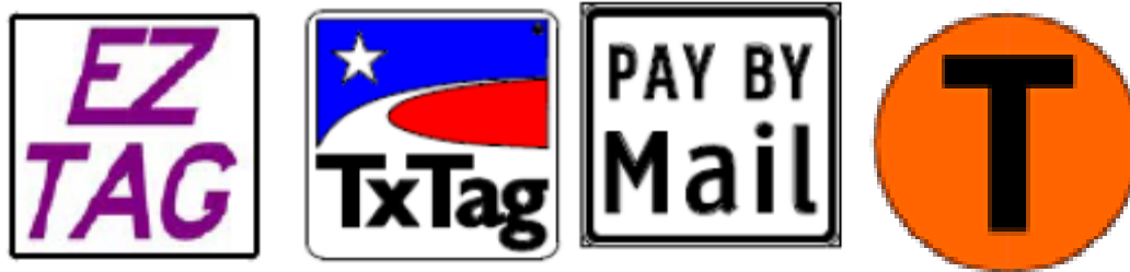
Figure 19. Payment plaques provided in TxDOT Draft Guidelines for Toll Roads and Managed Lane signing.
